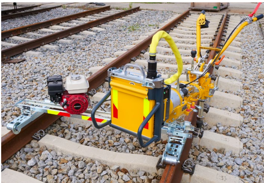
Fig. 8: The conversion kit for converting a machine with combustion engine enables battery-electric working without purchasing a new machine.
