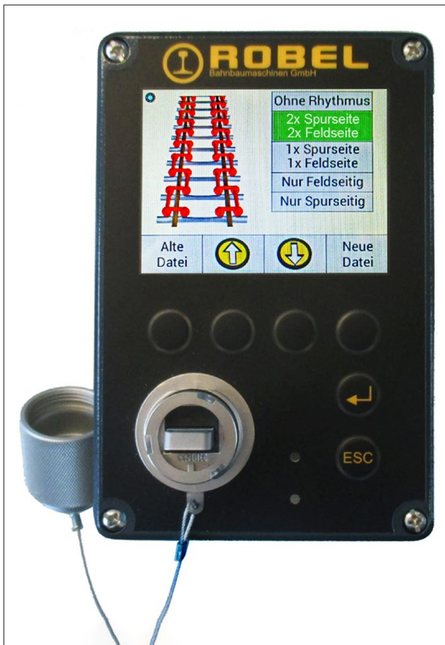
Fig. 4: The display shows the wrenching sequence inside / outside of rail, left / right rail.
