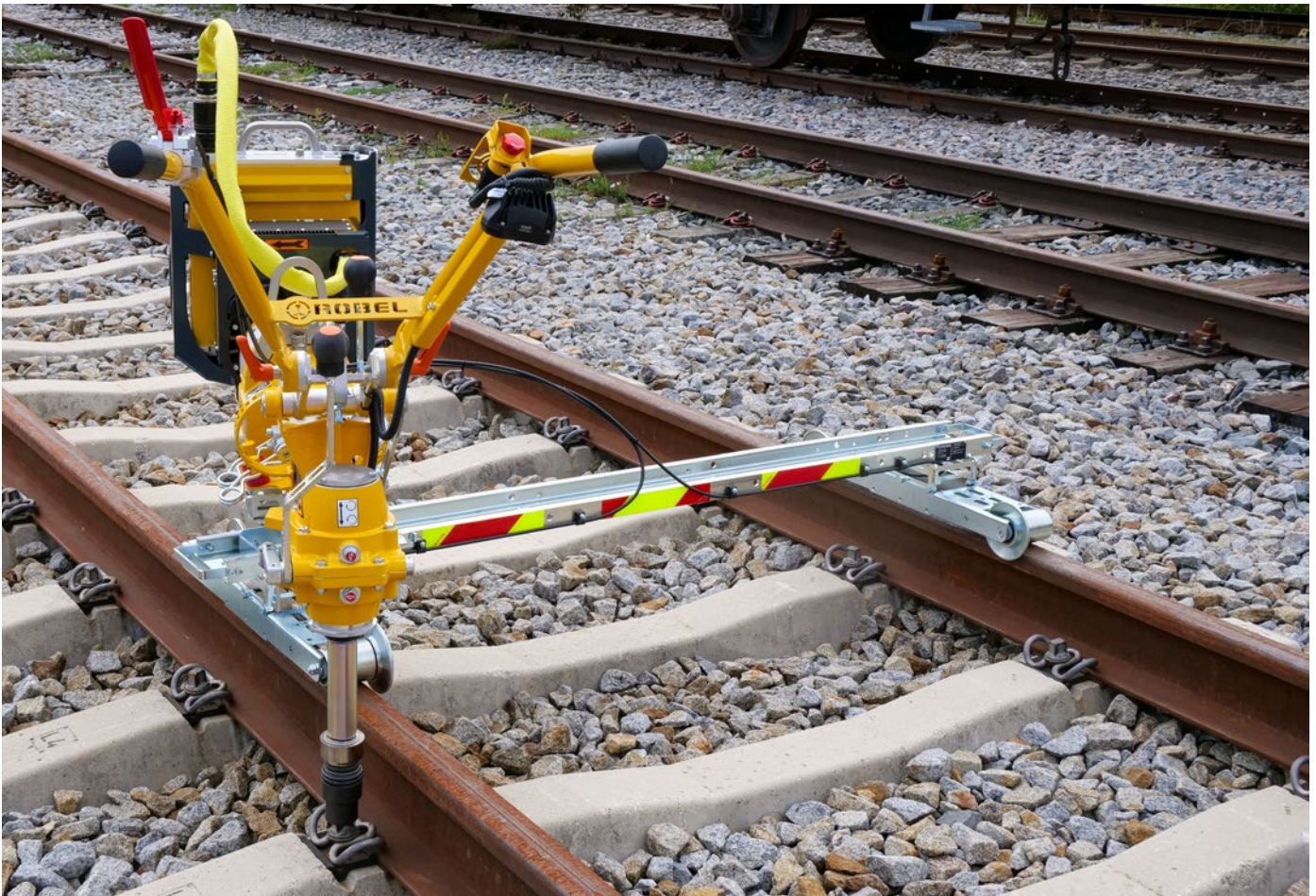
Fig. 7: The newly developed transverse bogie of the 30.82 HKS with connection to the dead man's handle.
