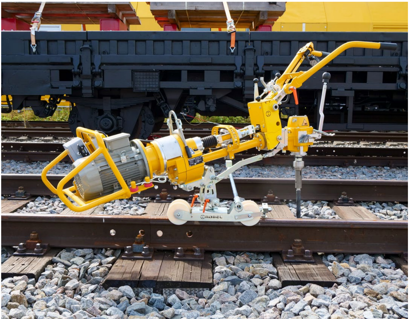
Fig. 9: Due to the parallelogram suspension, the tool of the combined power wrench and drilling machine 30.83 always stands vertically.
